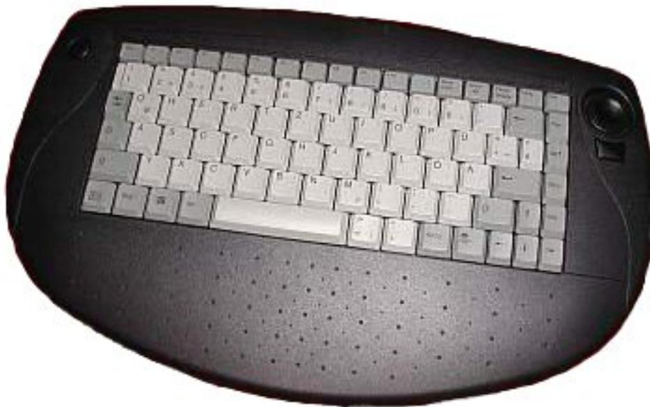
The keyboard events are intercepted by the front processor of the dBox, making it possible both to read the keyboard as a generic computer keyboard, and to interpret the keys as coming from a normal remote control.
